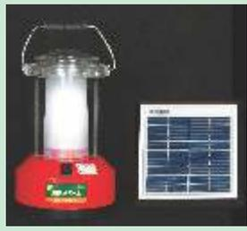
**Sun Grace** - A unique Dual mode brightness adjustable Solar Lantern with 2 high bright LEDs. In the first press of the switch, the light glows at 1/3 of its brightness to run for 12 hours and the second press at full brightness with more than 200 lumens covering 300 Sq. ft area for 6 hours. Comes with 3W solar module, 6V 4.5Ah battery and 2W LED load with optional electrical charging Adaptor. There are 3 indicators to show the condition of the battery.
